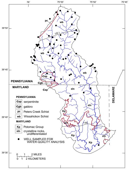
Figure 2. Generalized geology and location of wells sampled for water-quality analyses, Big Elk Creek Basin, Pennsylvania and Maryland.
